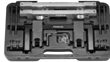
■ 912G5 P.1-21 Engine timing tool set for BMW N51/N52/N53/N54
