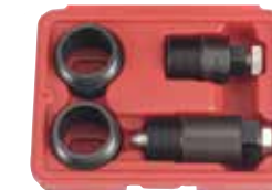
■ 904G7 P.1-80 Diesel injection pump puller (BMW)
